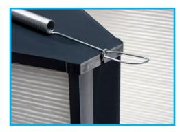
V-FORCE filters are made with four minipleat media packs fashioned into two V-shaped assemblies. The inset photo shows that the end panels are made with a notch to attach the spring latch used to secure the filter in the holding frame for reverse flow installations.
